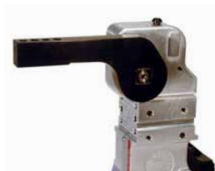
Lateral clamping arm, horizontal clamping position
