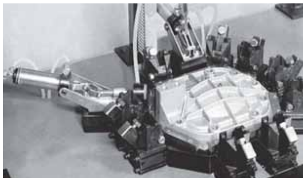
Power clamp models 871-2 and 803-MF on a pressure test fixture for vehicle gearbox lids
